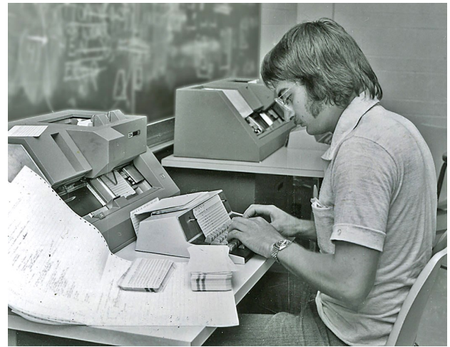
IBM Keypunch Machines Department of Computational Science Used with permission from the University of Saskatchewan © University of Saskatchewan Archives & Special Collections memorysask.ca/computers-computational-centre Photograph Collection, A-9767 (Photographer: Gibson)
