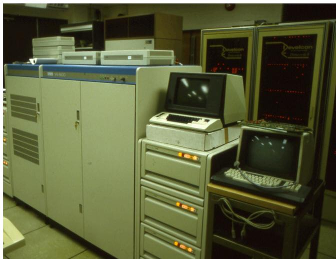
*Develcon Dataswitches in rear of photo, in Arts 70. Small boxes on top of VAX in foreground are first Ethernet concentrators to which terminals were connected to have access to the new Ethernet network, in 1985.*
