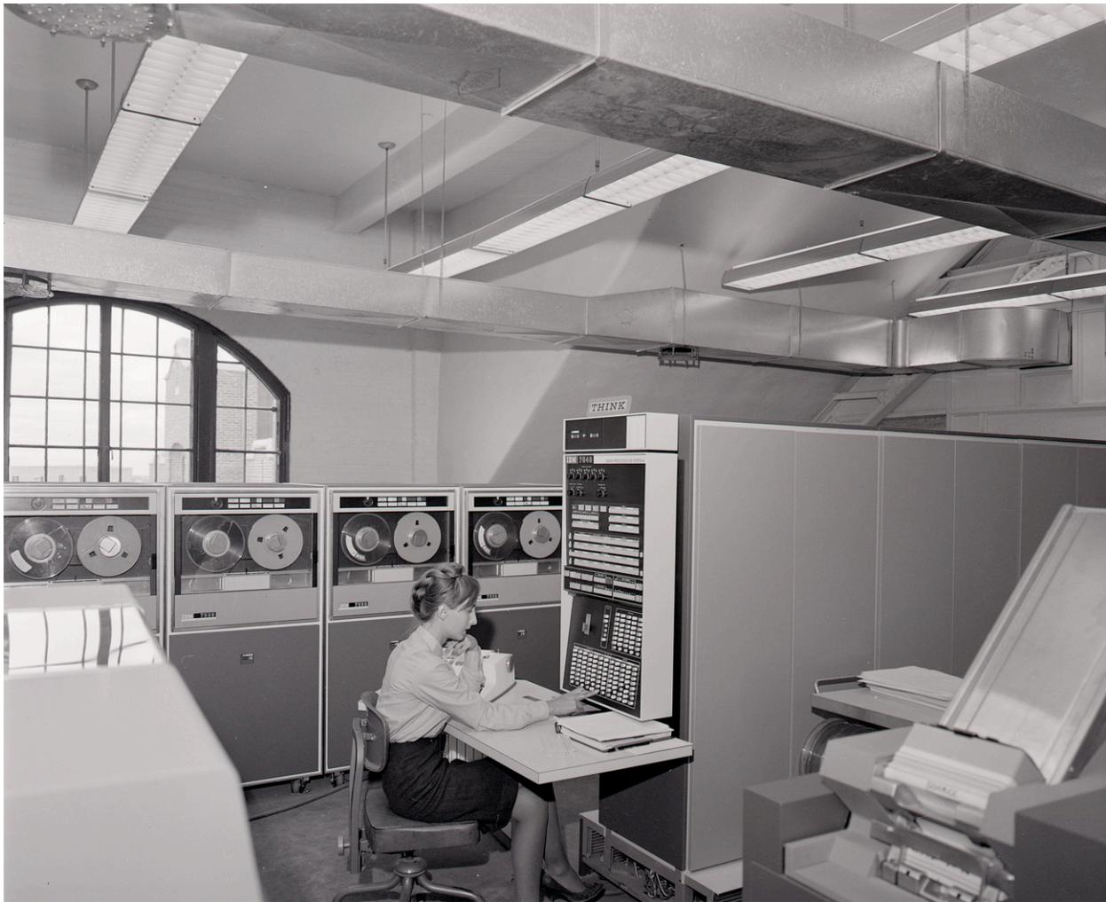
*The IBM 7040, the first 'mainframe' used by the University, installed in the Engineering Building in 1965. The card reader is front right, and in the left foreground is the side of the line printer, where all output was obtained. Several tape drives are shown in the background.*
