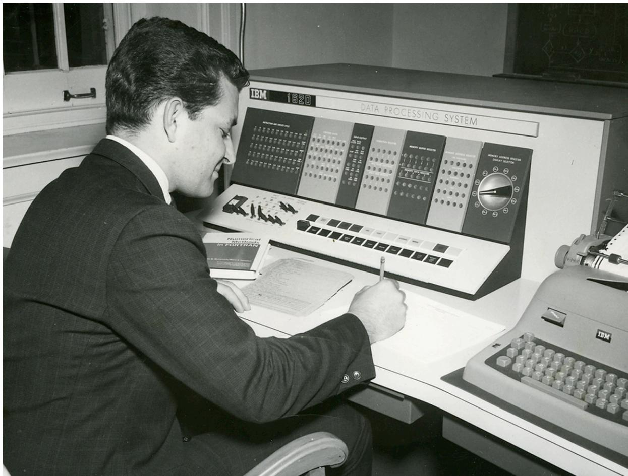
*The IBM 1620, installed in the Engineering Building in 1963. Note the amount of switches and knobs that the user had to manipulate to get a program activated.*
