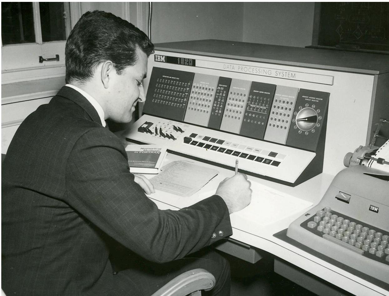
*The IBM 1620, installed in the Engineering Building in 1963. Note the amount of switches and knobs that the user had to manipulate to get a program activated.*
