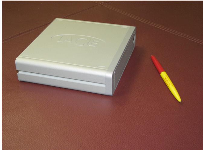
*500 Gbyte disk drive in 2007. Equivalent to almost 3,000 RP06 drives of 1979. Model courtesy of NeuralNet Interactive, Saskatoon.*
