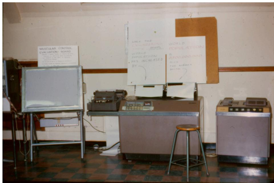
*The first digital computer on campus: the LGP-30 machine in the basement of the Crop Science Building, installed in 1957.*
