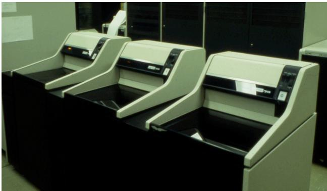
*Three DEC RP06 disk drives. Each one of these units, about the size of a household washing machine, held 175 Mbytes of information.*
